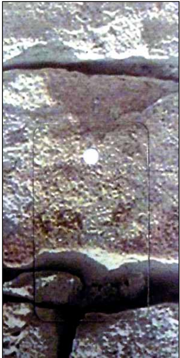
5,000 hours of Xenon accelerated exposure (central area) versus unexposed metal (outer area).
